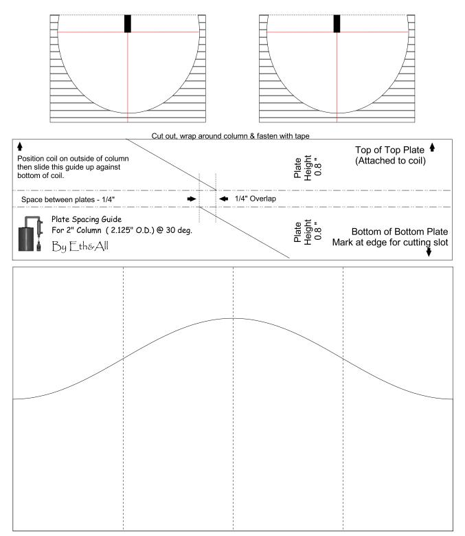
Above are two wrap-around templates that are very useful. The rectangle is divided into quadrants so that the thermometer tube location can be positioned 90° from the take-off tube. The other shows how the 30° slot will be cut in the column.
