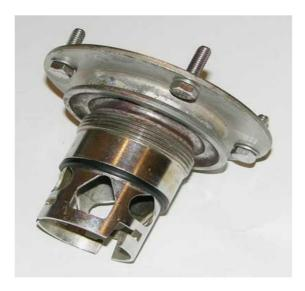
The tab is made of 3mm sheet metal, so you could tap holes and screw in screws. Then I cut the gasket visible below from the silicone sheet. Its thickness is 5mm
