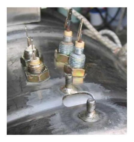
The use of two heaters has the advantage that it largely avoids the problems associated with home electrical system overload. The load of 3kW is over 13A,. However, it often happens that sockets are on 10A fuses. Then we simply disconnect the 1000W heater and work on the second o power of 2000W.
