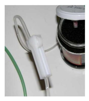
The ends of the hoses should be well weighted, which makes them easier to arrange.
