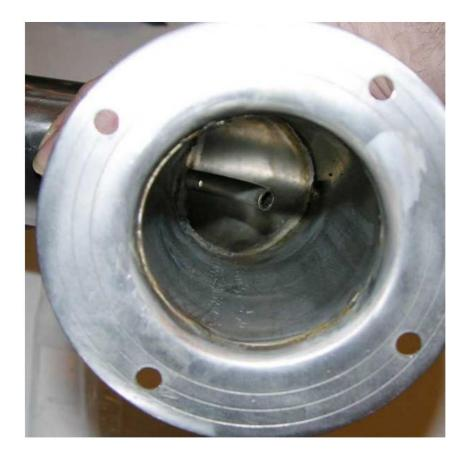
The condenser spiral is made of a 2.5m section of a DN12 corrugated pipe (smaller diameter 12mm, larger diameter 16mm).
