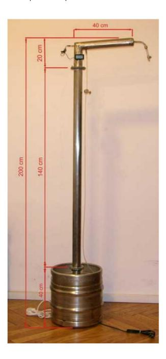
I will start describing the construction details from the heating container. I used a 30l keg for this
