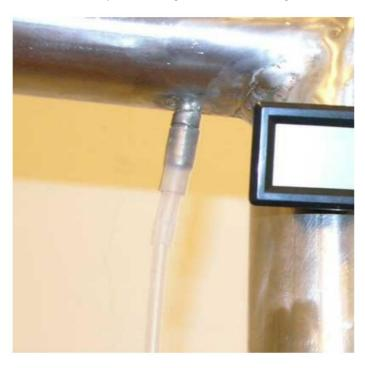
Such a thin tube has sufficient capacity and works very well with the pinch valve. Besides, it is much cheaper than the typical 9.0x1.5mm.
