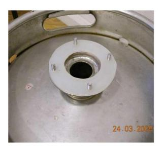
A second flange with appropriately drilled holes is welded to the main pipe. When assembled, the connector looks like this:
