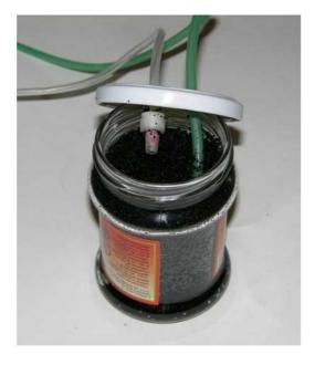
Holes should be made in the lid with a diameter slightly smaller than the silicon tubing.
