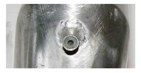
The pond dam is close to half the diameter of the pipe, but the return tube is welded low so that the pond it was as shallow as possible. In the photo below you can perfectly see the thermometer hole and the return tube hole.
