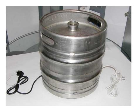
As heating elements, I used two 1000W and 2000W heaters
