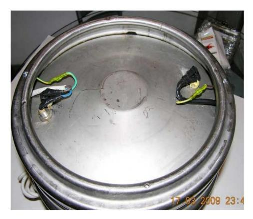
Perhaps protection with heat shrink tubing would be better than tape.
