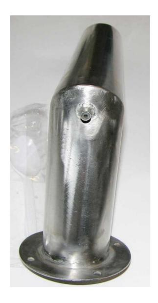
The thermometer mounting hole is made of a piece (about 15mm) of 8.0x1.0mm tube. In the middle there is pressed in gasket made of a piece of silicone tubing 6.0x1.5mm. The thermometer sensor falls into such a seal with quite a lot of resistance, so it is worth just slipping it before installation.
