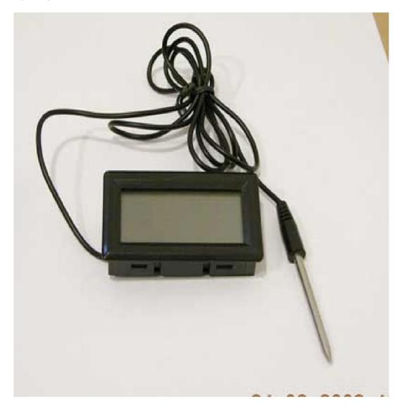
There is ST 9290 model c. Range: -50 ° C ~ + 150 ° C , accuracy:  $\ddot{y}$  1 ° C , resolution: 0.1 ° C Has an alarm, debt. 60cm cable. It costs about PLN 50
