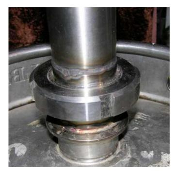
As I wrote before, the whole loudspeaker is made of a 60.3x2.0mm KO tube. Interestingly, the price is only slightly higher than the popular 52x1.5mm pipe. This is one of the reasons I chose it for construction of a model column. The second reason is the larger diameter that allows you to work with a power of 3kW. Attention! if the scourers are compacted too much, such a heating power may already flood the column of this diameter i prevent its proper functioning.
