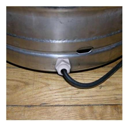
It is good to protect the wires with a special non-flammable insulating gland, available in any electrical store.
