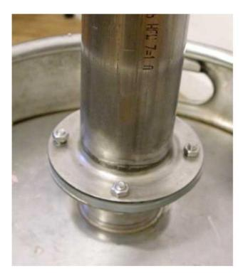
Of course, you can use a quick-SMS connector, but its price is about three times higher than the above solution. It is also difficult to access for diameters 60.3 mm. Below I present the SMS mount.
